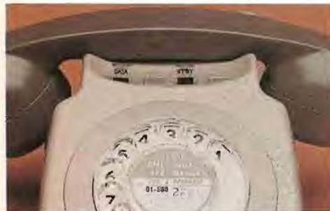
Fig T3 Telephone provided on installations consisting of a private circuit with speech facilities and a standby exchange line.
