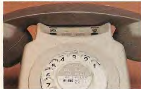
Fig T4 Exchange line telephone when not associated with a private circuit showing location of AUTO ANS button (when fitted).
