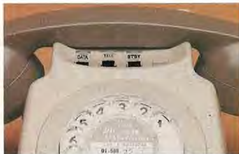
Fig S3 Private Circuit telephone when provided on an installation with a standby exchange line.
