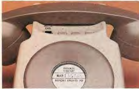
Fig T2 Private Circuit telephone showing typical position of 'CALL' button.
