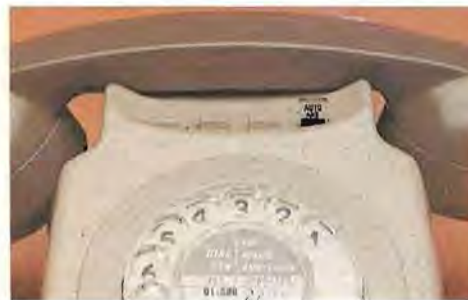
Fig R4 Exchange Line telephone when not associated with a private circuit, showing position of AUTO ANS button.
