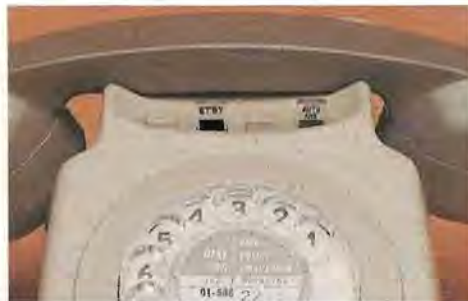
Fig R3 Exchange Line telephone when provided as a standby to a private circuit and where the terminal has automatic answering facilities.
