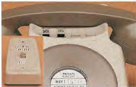
Fig S2 Private circuit telephone where speech facilities are provided. Inset shows alternative switch to 'DATA' button on telephone.
