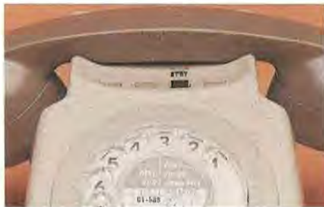
Fig R2 Exchange Line telephone when provided as a standby to a private circuit with alternative speech facilities.
